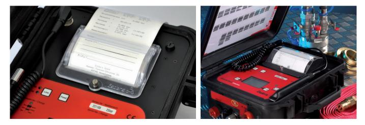
In order to get the advantages of a conventional barograph, a printer with a 112mm paper width is integrated into the box, which makes the current pressure trend recognisable in the form of a pressure curve. The illustrated pressure range can be freely selected, e.g. illustration from 5 to 7 bar. The measurement values can be recorded in a timecontrolled manner (e.g. every minute).
