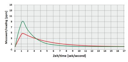
\* A comparison of the reaction time is carried out with the so-called T90 value. This value shows how many seconds it takes to reach 90% of the measured value.
